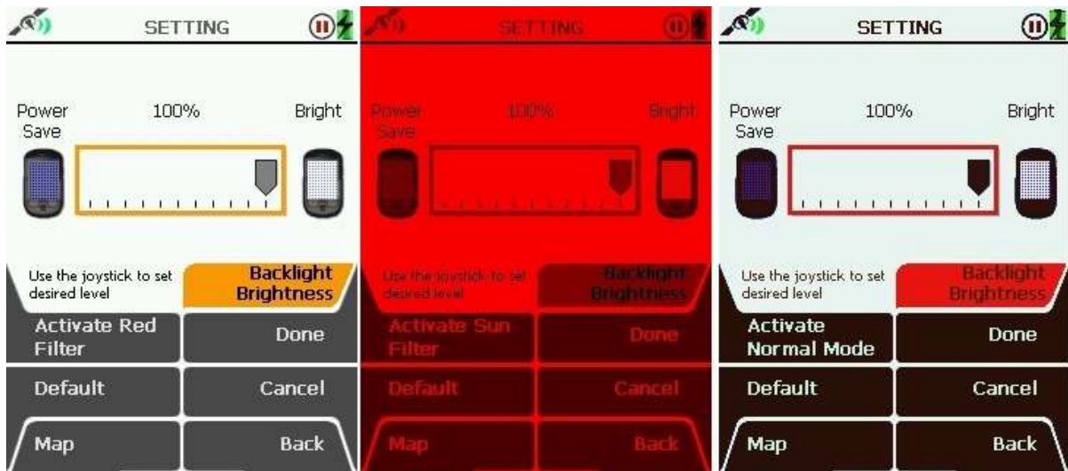
Figure 03: The normal mode (left), the red filter (centre) and sunlight filter (right).
