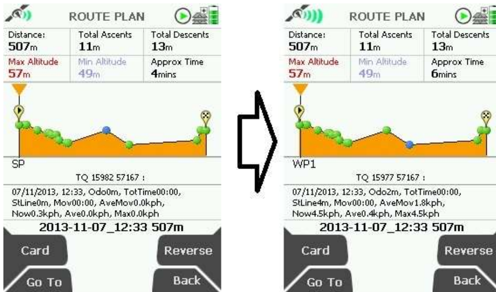
Figure 07 - On the left the position indicator (blue dot) is positioned centrally, as the walk continues the position indicator moved along the route line to the next indicated waypoint.
